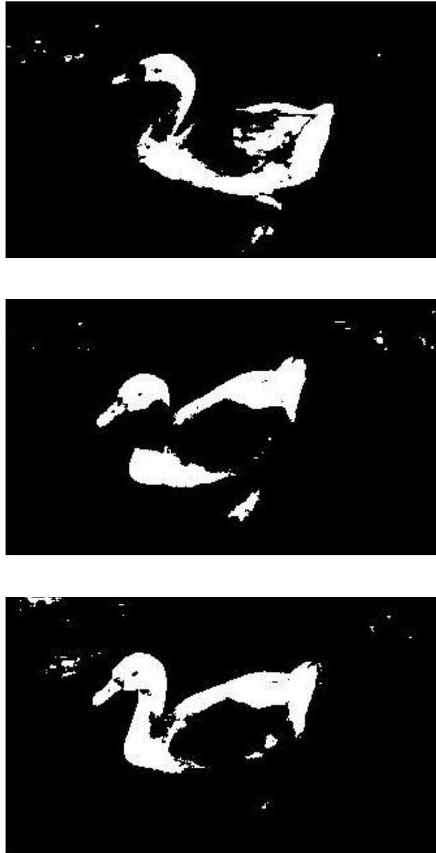
Fig 4.1 A sequence of frames obtained after applying approximate median filter background subtraction to a video
