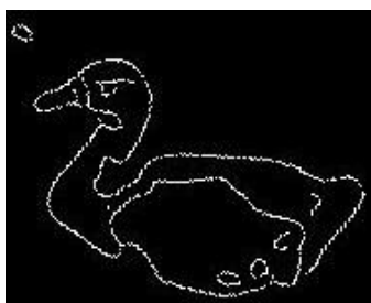
Fig 4.20 Result of Hough transform on binarized Canny edge detected image
